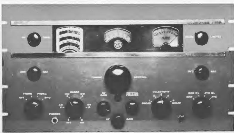
Figure 1: Front panel of the RCA-CR-91 general-purpose communications receiver. The AGC switch (extreme right) was subsequently modified to include "SSB" in a fifth position.
